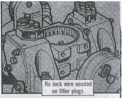
the steel vent plug stripped out the threads in the grip reservoir. That meant changing the reservoir.
