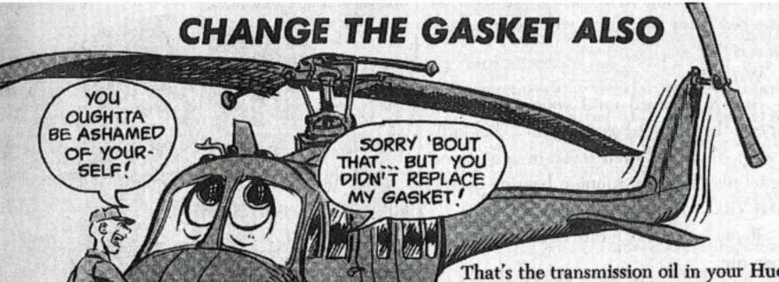
Drip . . . drip . . . drip. No, that's not a leaky water faucet. That's the transmission oil in your Huey (UH-1D/H) leaking—if you didn't use a new gasket when you changed the transmission's primary internal oil filter. That gasket's due for replacement every time you take the filter out. That's the word in para 7-9 of TM 55-1520-210-20 (Sep 71).
