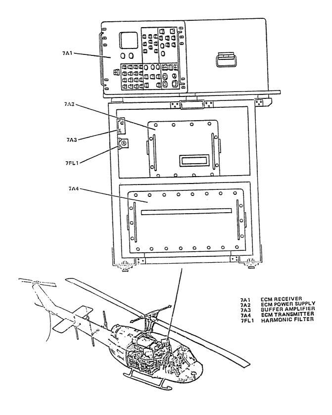
Figure 16-51 ECM Rack Equipment Locations, Unit 7
