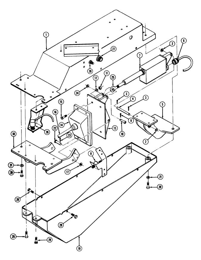
Figure 9-11. Forward Mission Antenna Mount, OE-201/ARQ-33 (Sheet 1 of 2)
