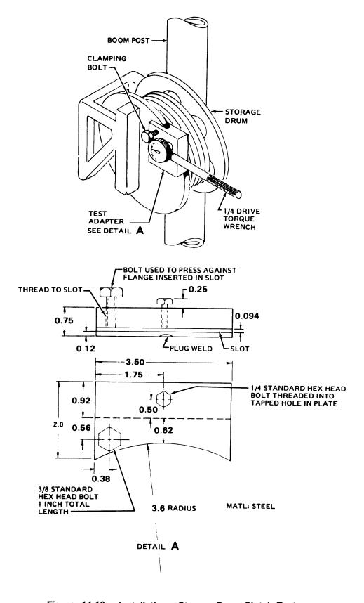
Figure 14-10. Installation - Storage Drum Clutch Tester
