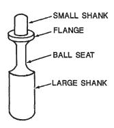
Figure 11-13.2. Pin 7 (PM 21217) Area Identification
