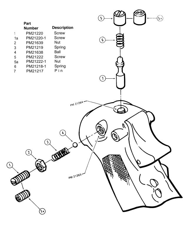
Figure 11-13.9 Exploded View of Trigger Detent Mechanism Components
