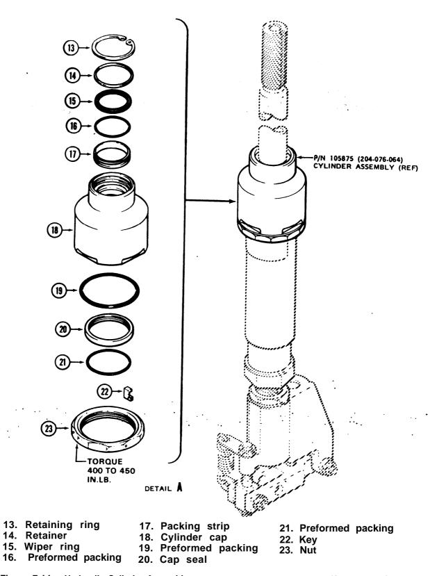
Figure 7-14. Hydraulic Cylinder Assembly — Disassembly and Assembly (Sheet 2 of 3)
