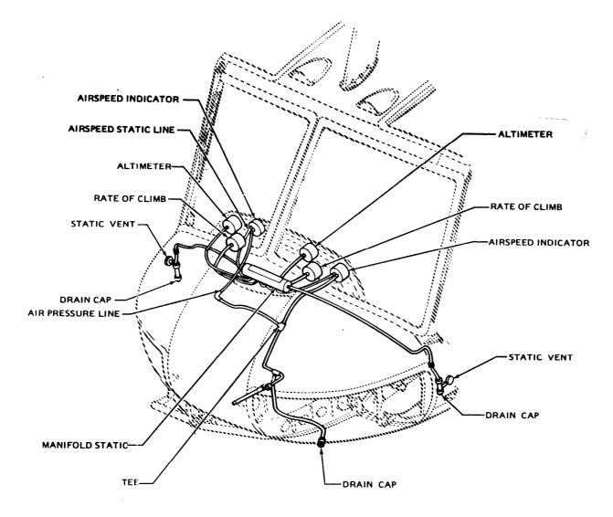
Figure 8-1. Instrument Piping (Nose-Mounted Pitot Tube) (Sheet 2 of 2)
