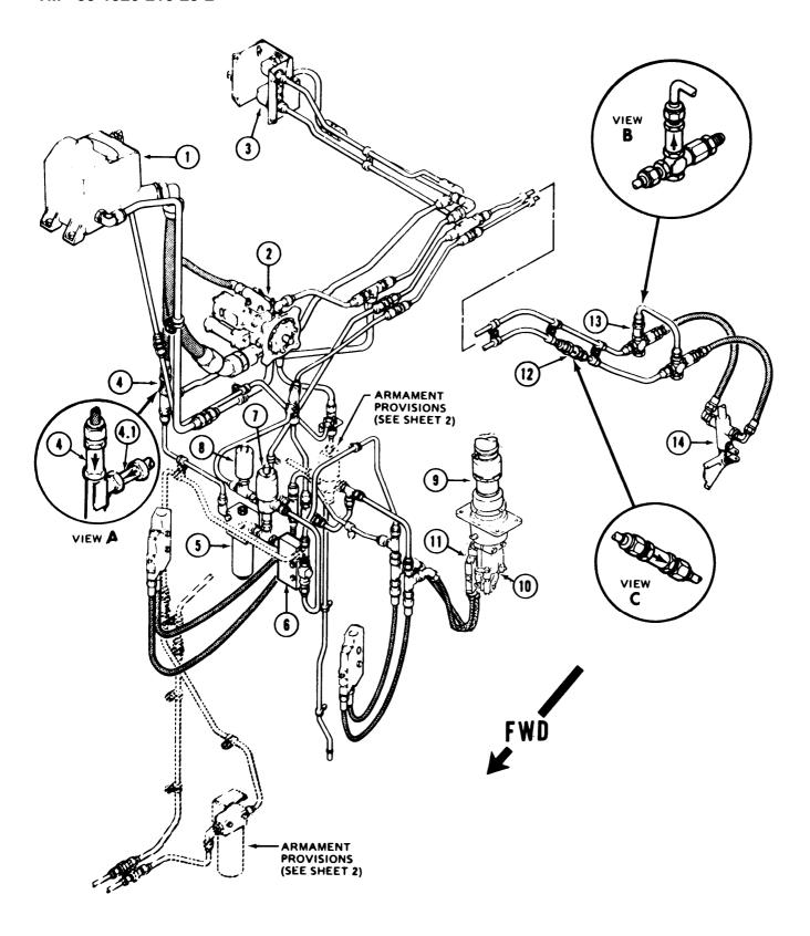
Figure 7-1. Hydraulic System — Flight Controls (Sheet 1 of 2)
