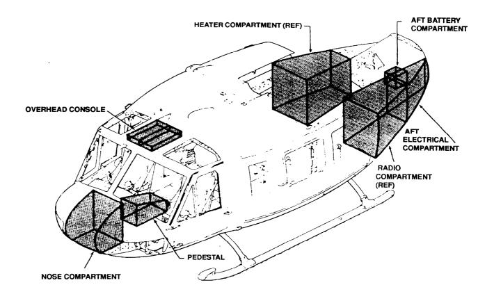
Figure 9-1. Compartment Location - Electrical
