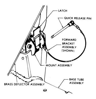
Figure 16-28. Brass Deflector Assembly — Right Side Shown
