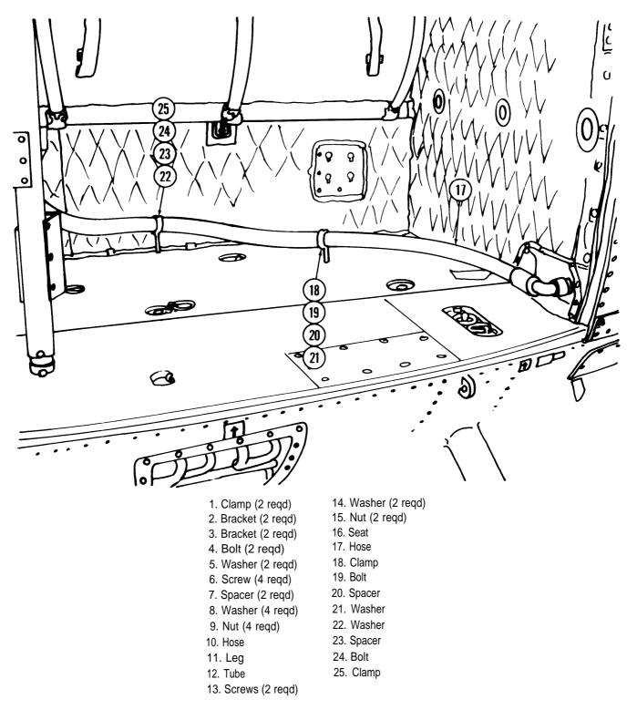
Figure 16-8. Vent Hose Installation (sheet 2 of 2)
