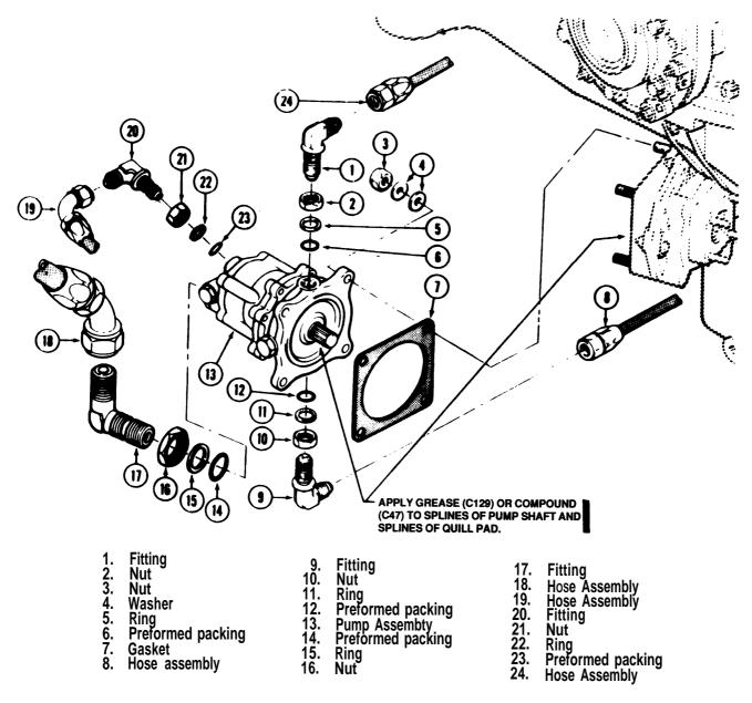
Figure 7-4. Hydraulic Pump Removal Installation
