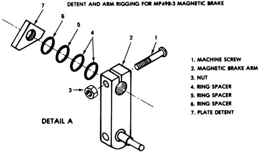
Figure 11-15 Magnetic Brake Adjustment (Sheet 1 of 2).
