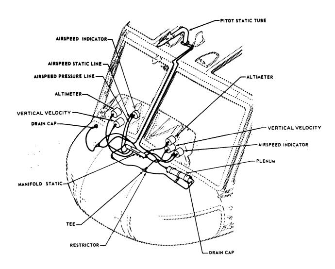
Figure 8-1. Instrument Piping (Roof-Mounted Pitot Tube) (Sheet 1 of 2)
