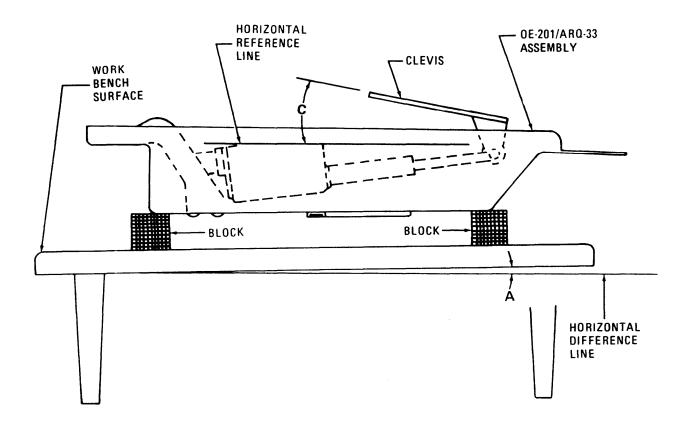
Figure 9-14. Antenna Mount Assembly Extended Limited Switch Bench Setup
