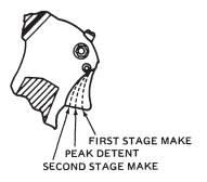
Figure 11-13.5. Approximate Trigger Position
