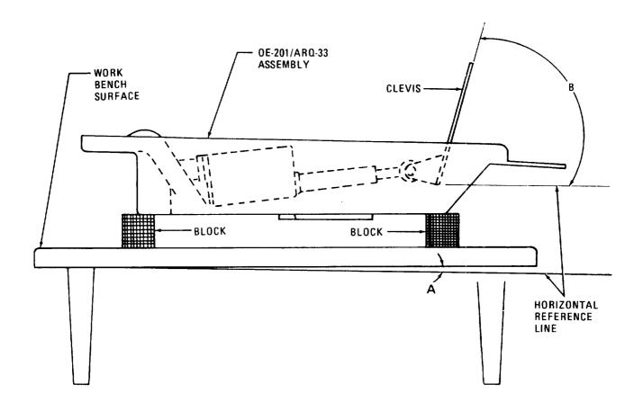
Figure 9-13. Antenna Mount Assembly Retract Limit Switch Bench Setup
