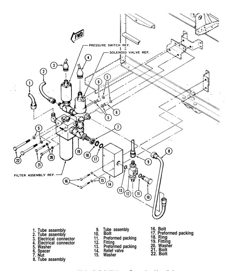
Figure 7-6. Hydraulic Relief Valve — Removal and Installation
