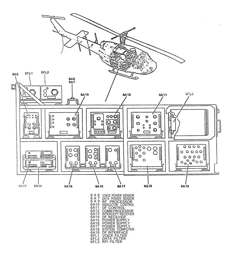
Figure 16-49 Base Rack Equipment Locations (side view), Unit 6
