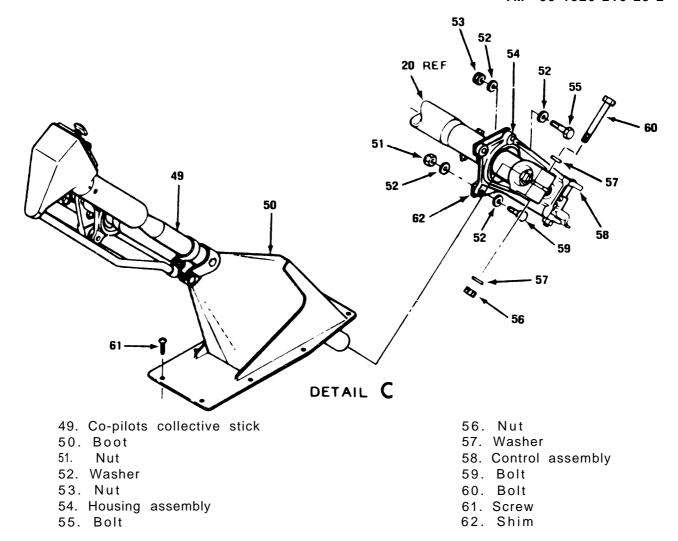
Figure 11-2. Collective Jackshaft (Sheet 3 of 3)
