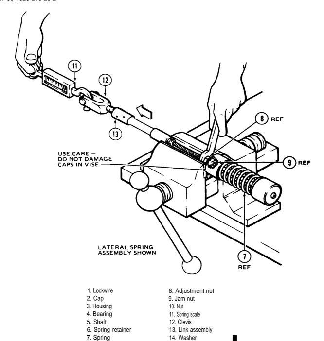
Figure 11-16. Force Gradient Assembly Adjustment (Sheet 2 of 2)
