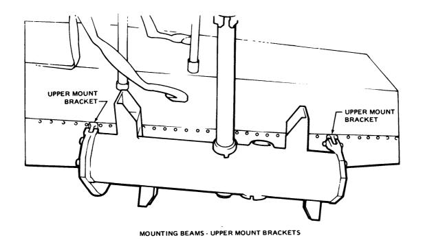
Figure 16-21. Armament Subsystem M23 Mount — Left Side
