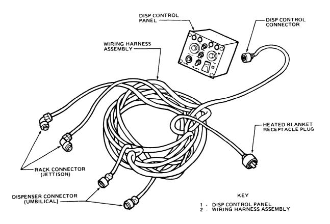
Figure 16-30. M56 Wiring Harness Assembly
