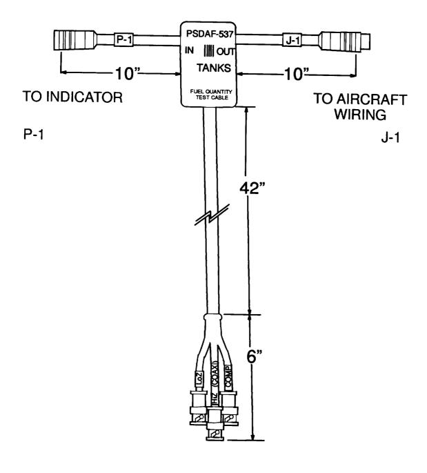
Figure 6-7.2 Fuel Quantity "T" Cable P/N PSDAF-537
