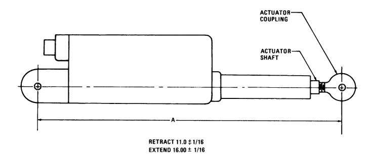
Figure 9-12. Actuator Pre-Installation Measurements
