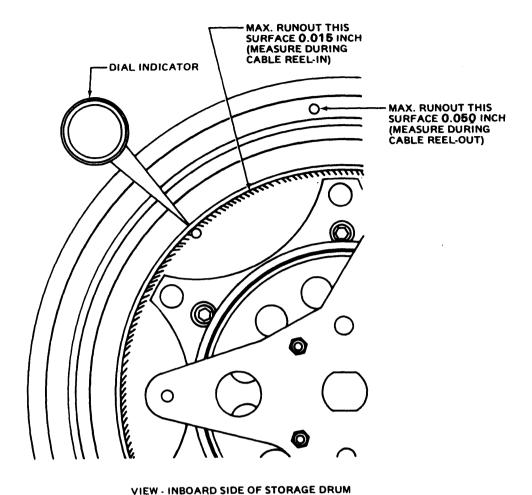
Figure 14-11. Measuring Storage Drum Runout
