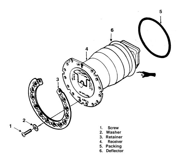
Figure 10-12. Closed Circuit Refueling Receiver (MMO 55-1520-210-30-55).
