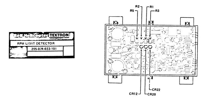
Figure 9-8A. BHT Model 205-074-033-101 Rpm Limit warning Detector
