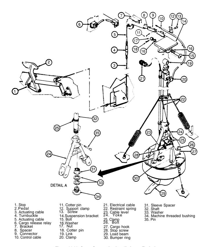
Figure 14-32. Cargo Suspension Installation — Typical
