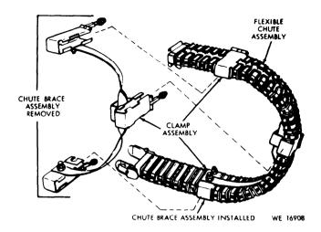
Figure 16-14. Installation or Removal of Brace Assembly or Chute Assembly
