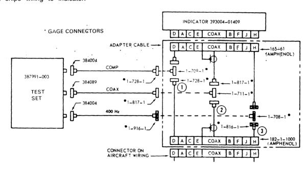
Figure 8-7. Circuit Arrangement and Adapter Cable for Adjustment Procedures (Crashworthy)
