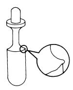
Figure 11-13.6 Burr Worn Up On Pin 7 (PM 21217)
