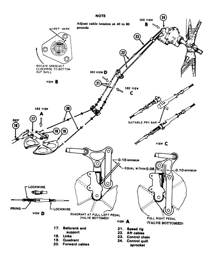
Figure 11-24. Tail Rotor Control System (Sheet 2 of 2)
