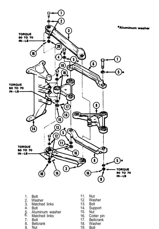
Figure 11-19. Mixing Lever Assembly — Cyclic Controls — Disassembly and Assembly
