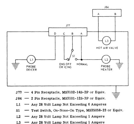
Figure 9-3. Icing System Test Box Schematic
