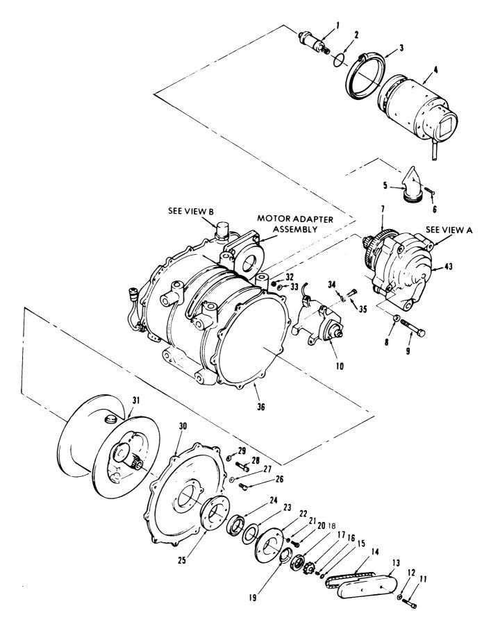
Figure 14-28. Winch Assembly (Sheet 1 of 2)
