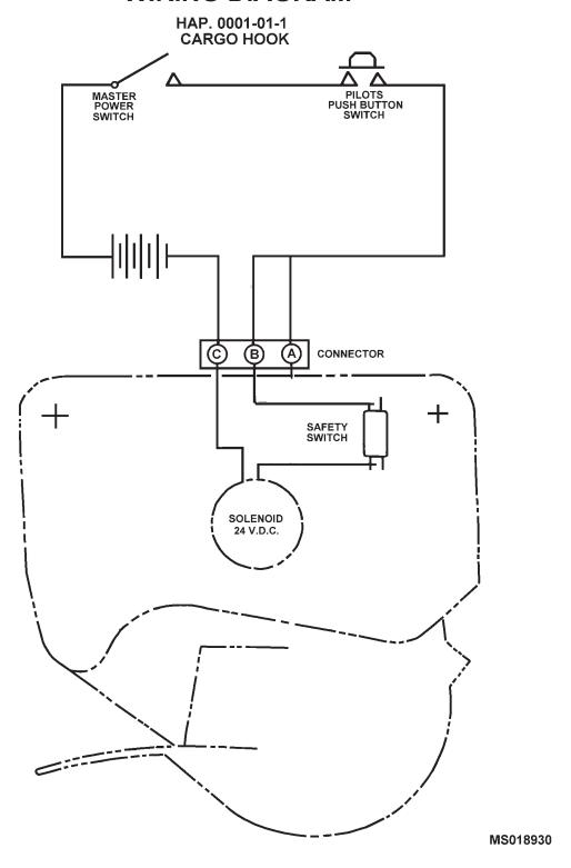
Figure 14-33.2. Wiring Diagram
