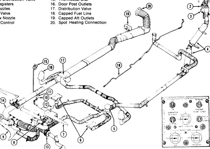
Figure 13-1. Heat-Defrost Air System without Auxiliary Heater (Serial Numbers 62-12351 thru 64-13901) (Sheet 1 of 3)
