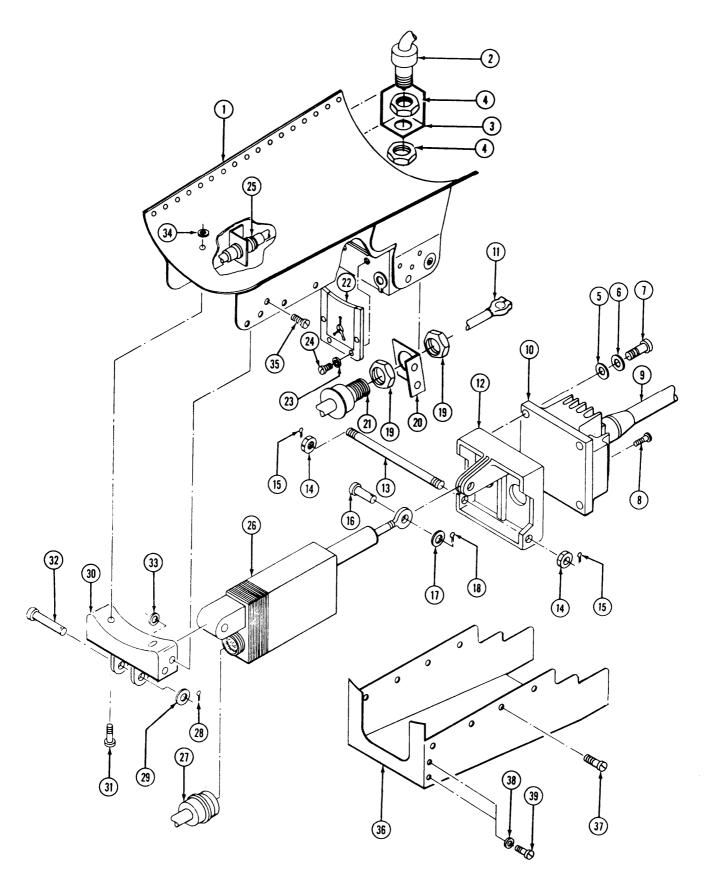
Figure 9-16. Antenna Mount Assembly, OE-202/ARQ-33 and OE-330/ALQ-151 (Sheet 1 of 2) 9-116
