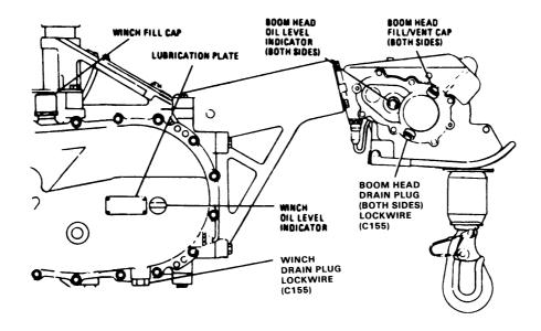
Figure 14-17. Oil Level Indicators and Drain Plugs
