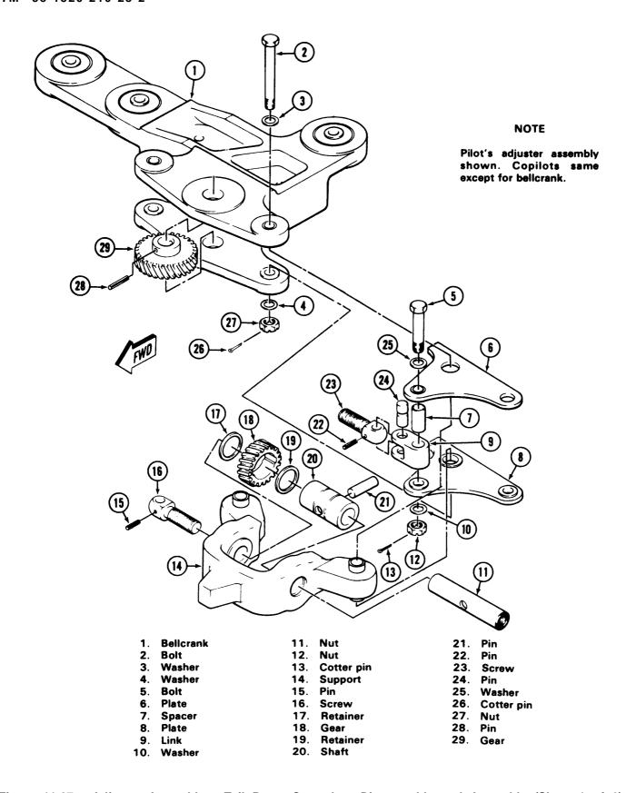
Figure 11-27. Adjuster Assembly - Tail Rotor Controls - Disassembly and Assembly (Sheet 1 of 2)
