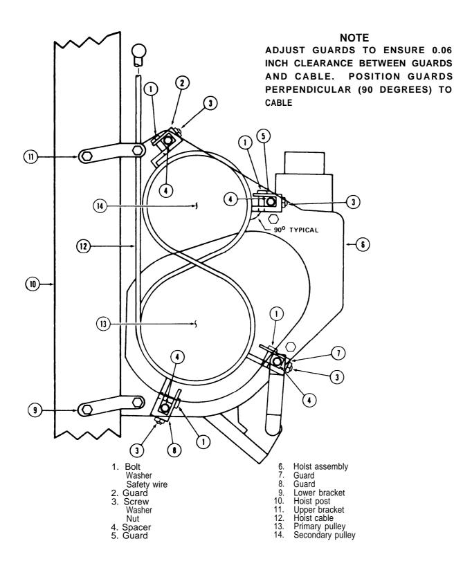
Figure 14-8. Cable Guard Installation
