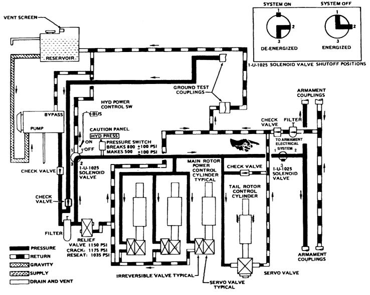
Figure 7-2. Hydraulic System Schematic (Gravity Feed) (Sheet 1 of 2)
