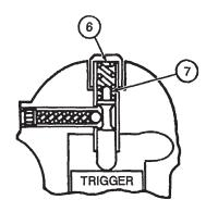
Figure 11-13.1. Internal Position of Trigger Detent Mechanism Components for "First Stage Make"
