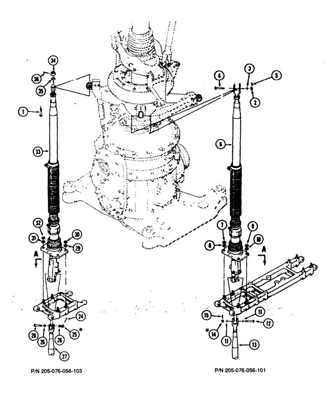
Figure 7-11. Hydraulic Cylinder Assembles Fore and Aft and Lateral Cyclic Controls-Removal and Installation (Sheet 2 of 4)
