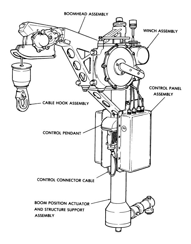
Figure 14-15. Rescue Hoist Assembly, General View.
