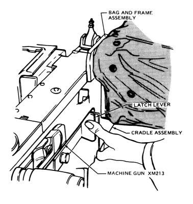
Figure 16-25. Installation/Removal of Bag and Frame Assembly
