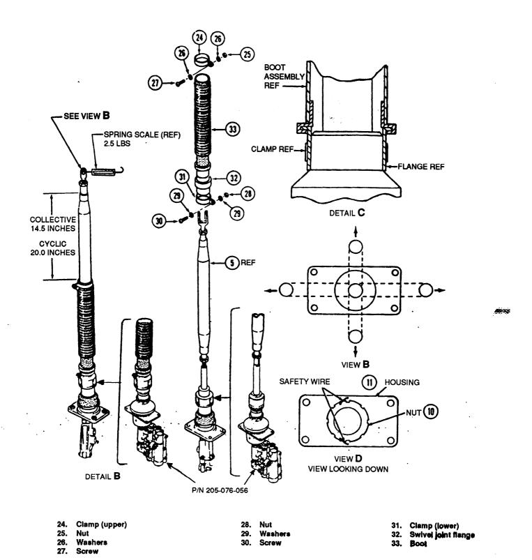
Figure 7-14. Hydraulic Cylinder Assembly - Disassembly and Assembly (Sheet 3 of 3)
