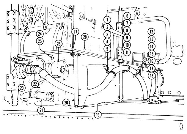
1. Clamp 15. Screw 16. Washer (2 reqd) 2. Clamp 17. Nut 3. Screw 18. Spacer 4. Washer 19. Oil Tank 5. Nut 20. Hose 6. Clamp 7. Clamp 21. Hose 8. Bracket 22. Coupling 9. Screw (2 reqd) 23. Coupling 10. Washer (2 reqd) 24. Washer (4 reqd) 11. Nut (2 reqd) 25. Bolt (4 reqd) 12. Clamp 26. Pump 13. Bracket 27. Screw (3 reqd, typical 4 places) 14. Screw 28. Seat
