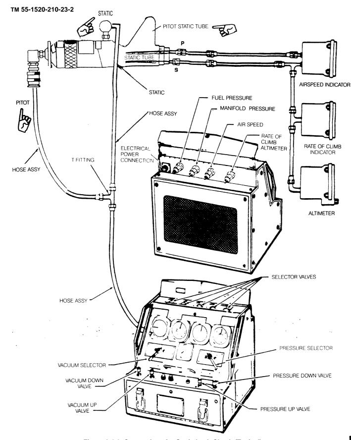
Figure 8-1.2. Connections for Static Leak Check (Typical)
