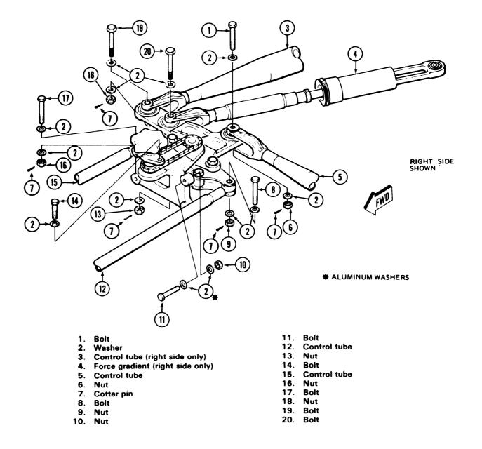
Figure 11-26. Adjuster Assembly — Tail Rotor Controls — Removal and Installation — Typical
