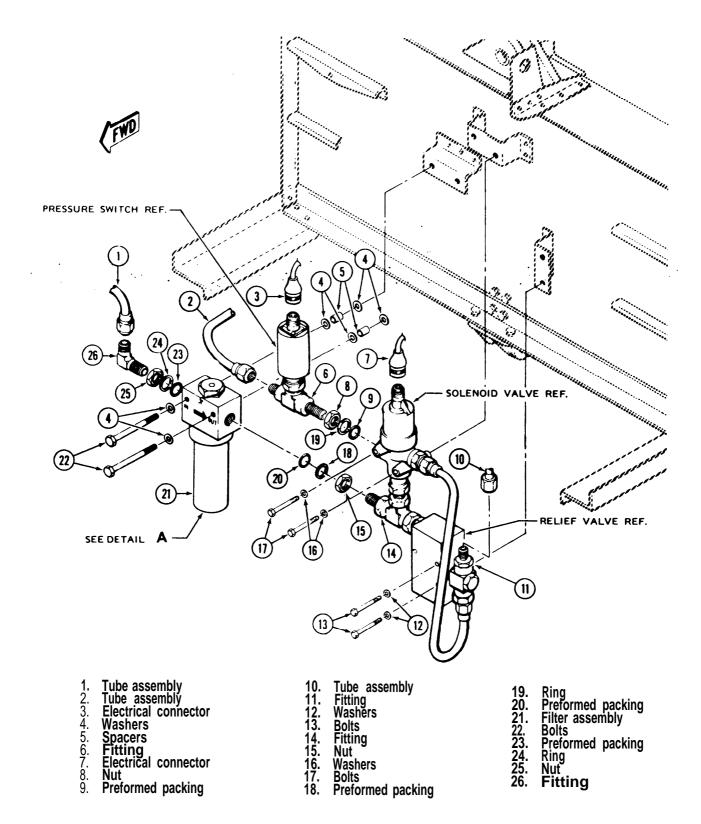
Figure 7-7. Hydraulic Filter Assembly – Removal and Installation (Sheet 1 of 2)
