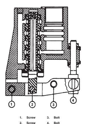
Figure 7-13. Hydraulic Cylinder Servo Valve (Wire Drive Type)
