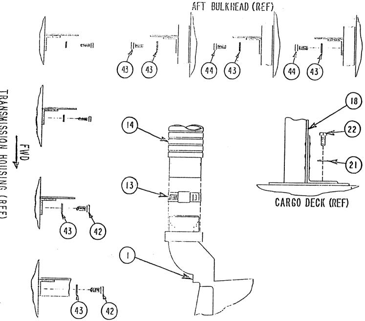
Figure 16-52 Navigation System AN/ASN-86; Removal and Repalcement aircraft Attach Points (Sheet 3 of 5) TRANSMISSION HOUSING (REF)
