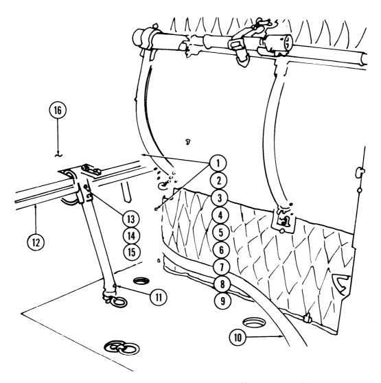
Figure 16-8. Vent Hose Installation (Sheet 1 of 2)
