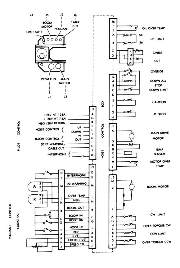
Figure 14-19. Control Panel Assembly, Controls and Indicators (Sheet 2 of 5)
