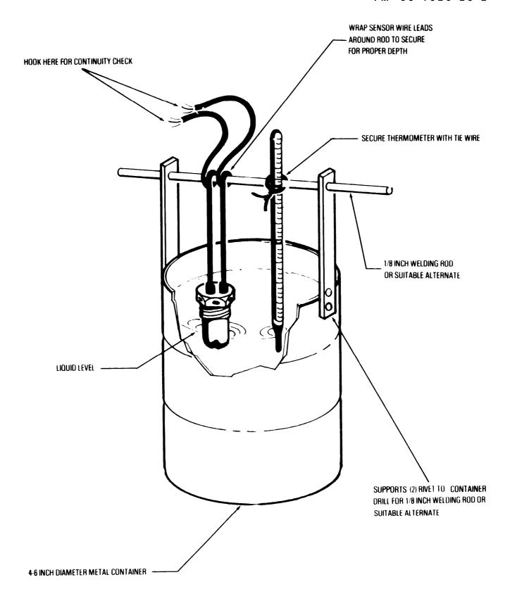
Figure 13-6. Setup For Heat Sensor Test
