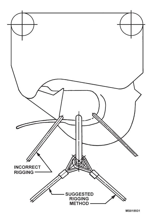
Figure 14-33.1. Rigging Method
