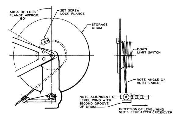
Figure 14-6. Hoist Cable to Storage Drum Attachment
