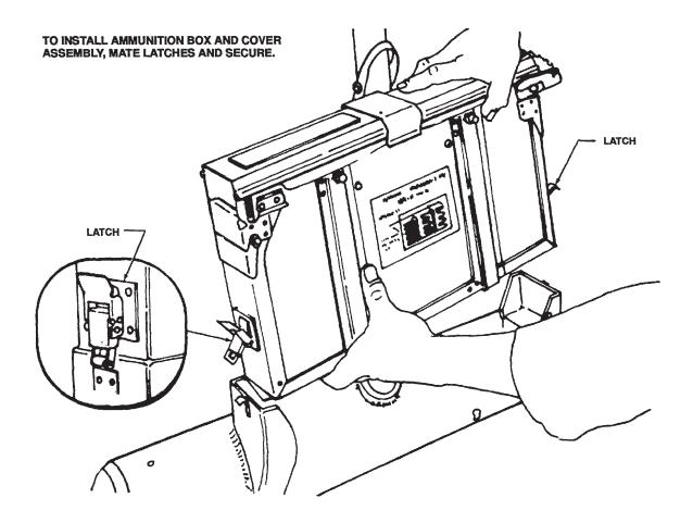
Figure 16-19. Ammunition Box and Cover Assembly—Removal
