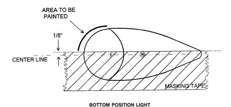
Figure 9-10.1 Position Light Lens Modifications
