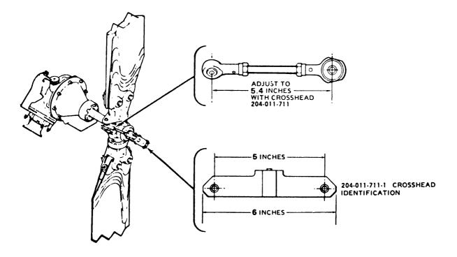
Figure 11-25. Tail Rotor Control Crosshead and Link Usage
