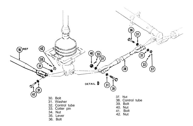
Figure 11-21. Cyclic Control System (Bellcranks, Levers, Supports, and Control Tubes) — Removal and Installation (Sheet 3 of 5)
