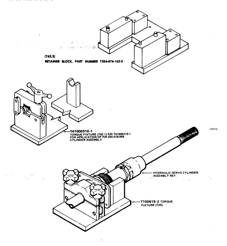
Figure 7-17. Tool Application Hydraulic Cylinder Assembly Supported in T100619-2 or T41000310-1 or T204-076-162-3 Torque Fixture
