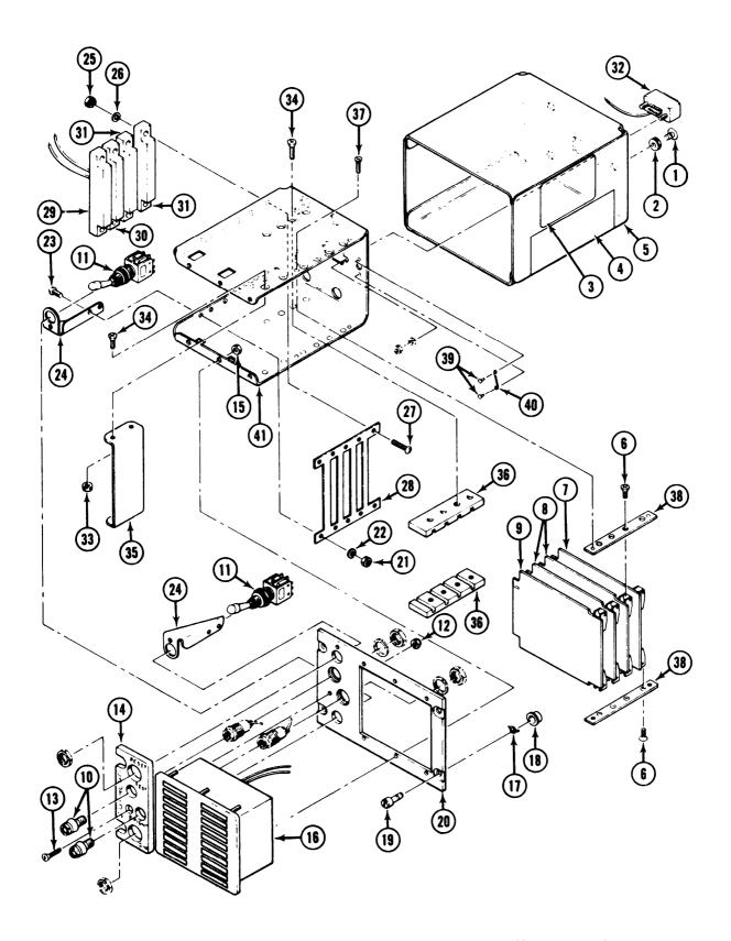
Figure 9-5. Master Caution Panel — Exploded View (Sheet 1 of 2)
