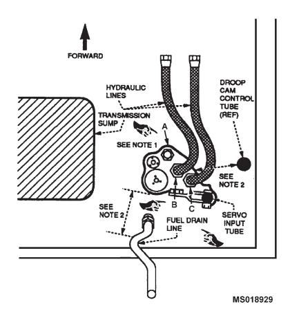
Figure 7-23.2. Position of servo, P/N 205-076-056-105, in collective position, looking up into hell hole
