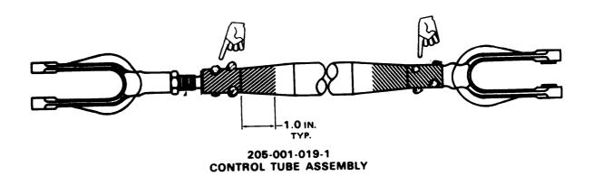
Figure 11-42. Wear and Damage Limits (Control Tubes Elevation Control System) (Sheet <sup>1</sup> of 2)
