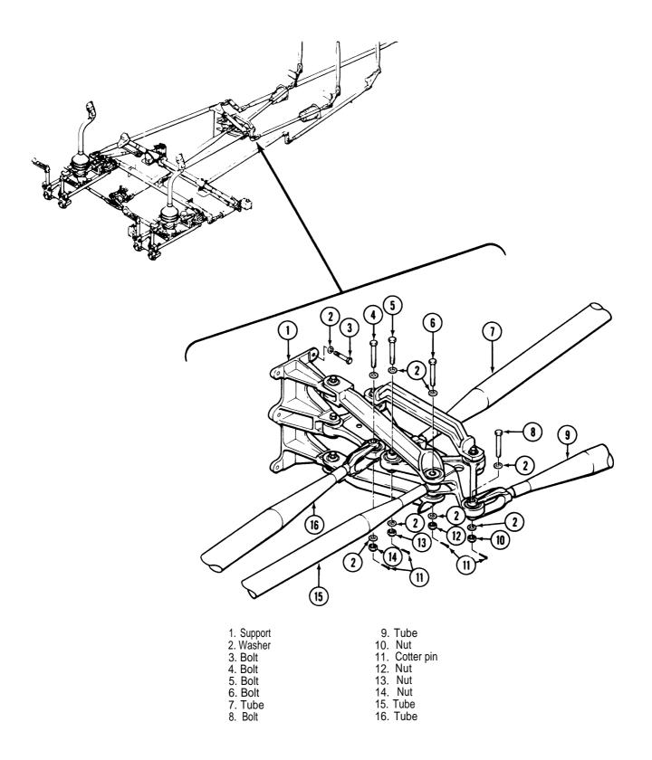
Figure 11-18. Mixing Lever Assembly — Cyclic Controls — Removal and Installation
