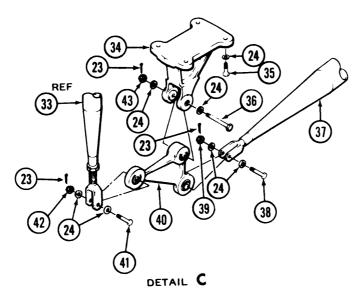
Figure 11-41. Elevator Controls System (Bellcranks, Levers, Supports, and Control Tubes) - Removal and Installation (Sheet 3 of 5)
