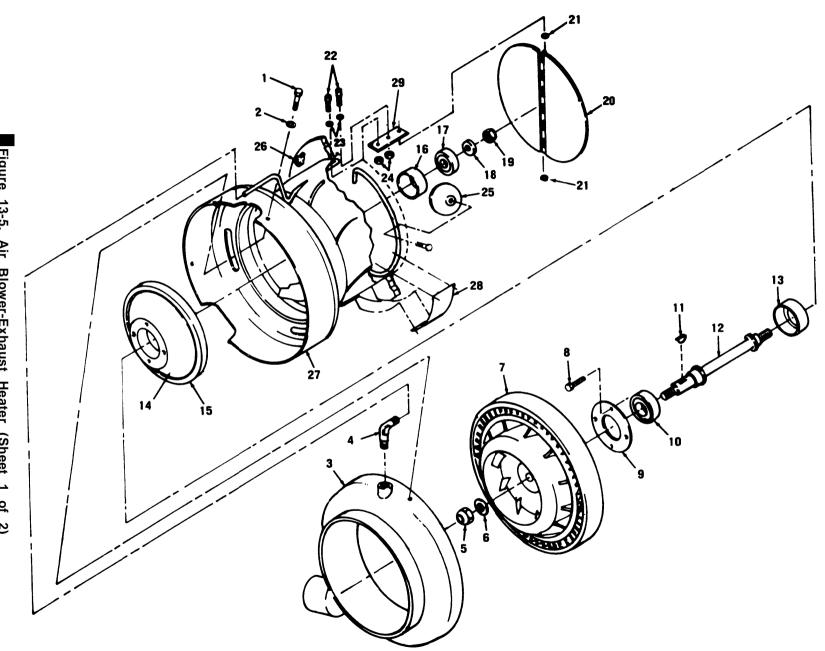
Figure 13-5. Air Blower-Exhaust Heater (Sheet 1 of 2)
