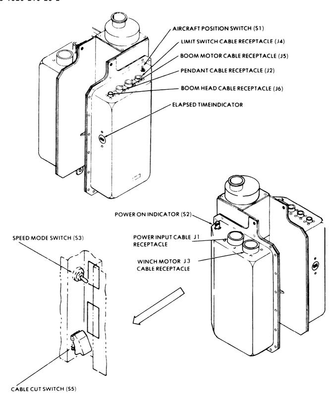
CONTROL PANEL (ROTATED 180 FOR CLARITY)
