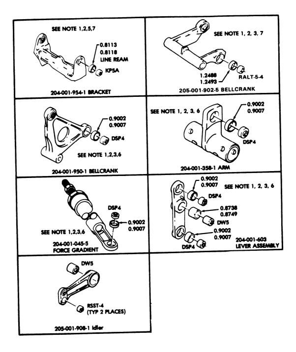
DSP4 Bearing Radial 0.012 Axial 0.030 DW5 Bearing Radial 0.005 Axial 0.030 DSP5 Bearing Radial 0.012 Axial 0.030 RALT 5-4 Bearing Radial 0.012 Axial 0.030
