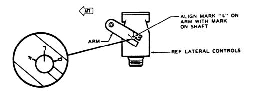
Figure 11-15. Magnetic Brake Adjustment (Sheet 2 of 2)
