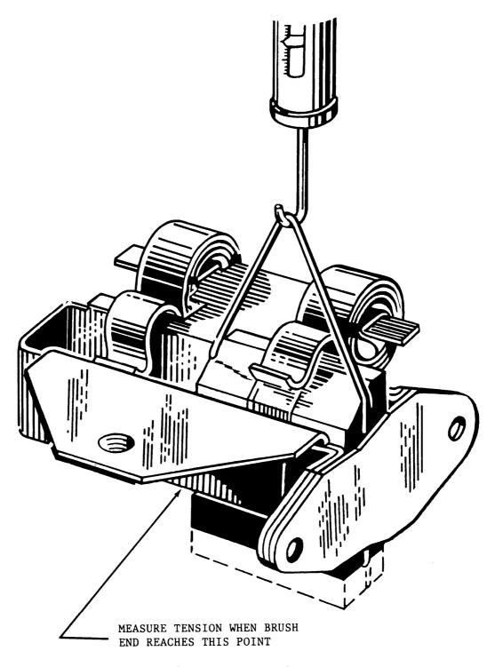
Figure 9-2.1.1 Checking Brush Spring Tension.
