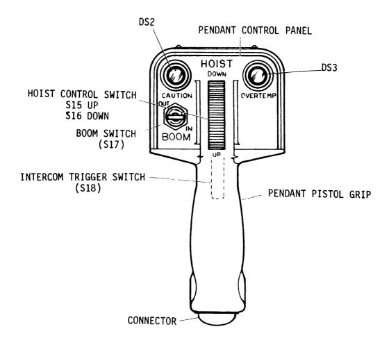
Figure 14-18. Control Pendant Assembly Controls and Indicators
