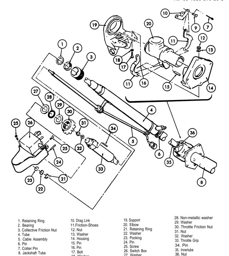
Figure 11-6. **Pilots Collective Stick Exploded View**
