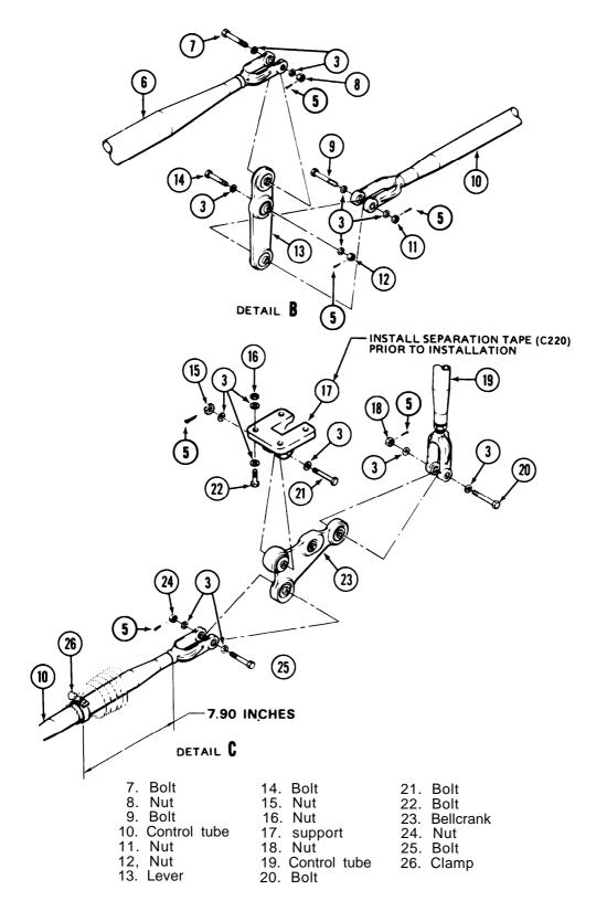
Figure 11-8. Collective Control System (Bellcranks, Levers, Supports, and Control Tubes) — Removal and Installation (Sheet 2 of 2)
