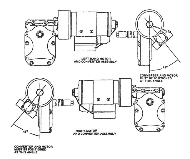
Figure 12-7. Motor and Converter Assembly — Left & Right Configuration
