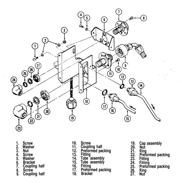
Figure 7-5. Hydraulic Test Connections — Removed and Installed
