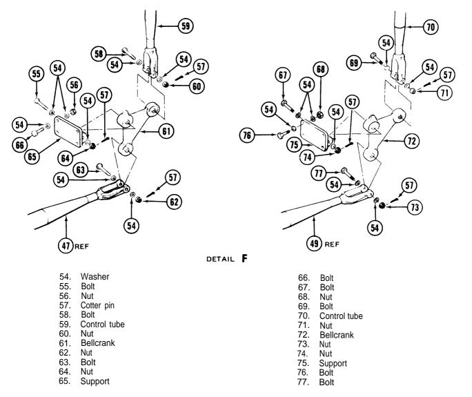
Figure 11-21. Cyclic Control System (Bellcranks, Levers, Supports, and Control Tubes) – Removal and Installation (Sheet 5 of 5)
