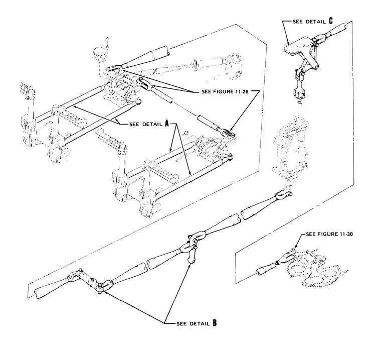
Figure 11-37. Tail Rotor Control System (Bellcranks, Levers, Supports, and Tubes) – Removal and Installation (Sheet 1 of 3)
