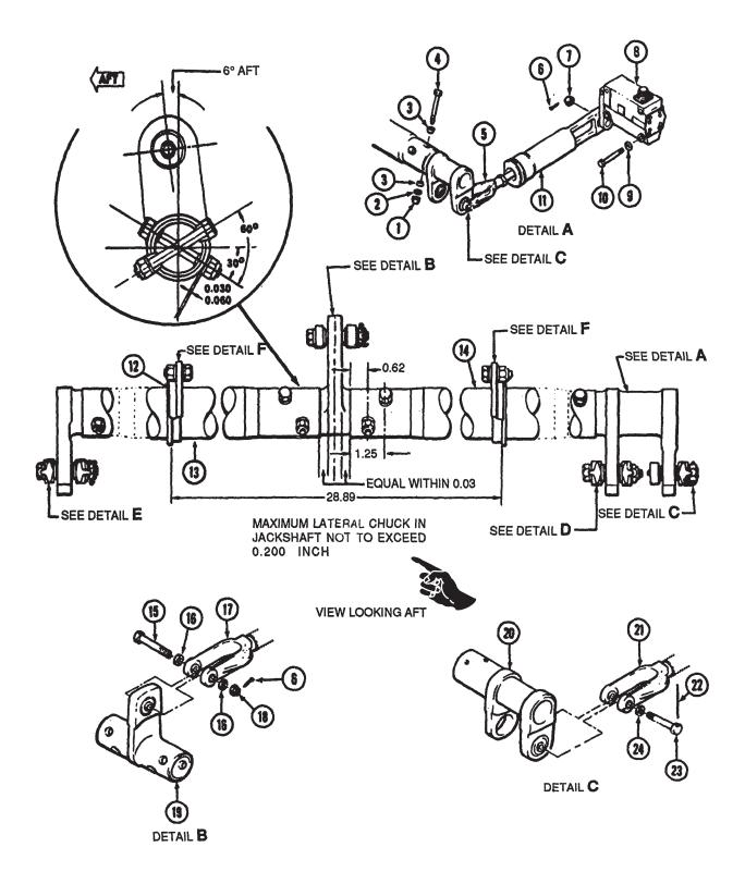
Figure 11-14. Cyclic Control Tube and Lever Assembly (Sheet 1 of 2)
