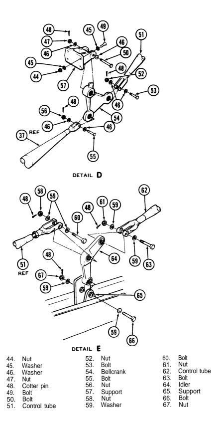
Figure 11-41. Elevator Controls System (Bellcranks, Levers, Supports, and Control Tubes) – Removal and Installation (Sheet 4 of 5)
