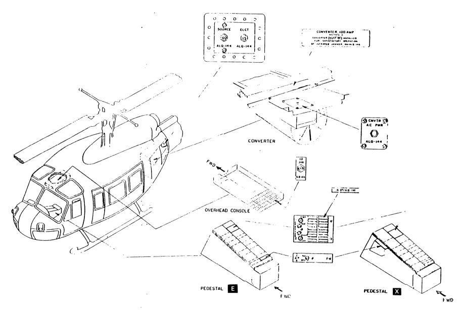
Figure 8-10. Radar Countermeasures System AN/ALQ-144
