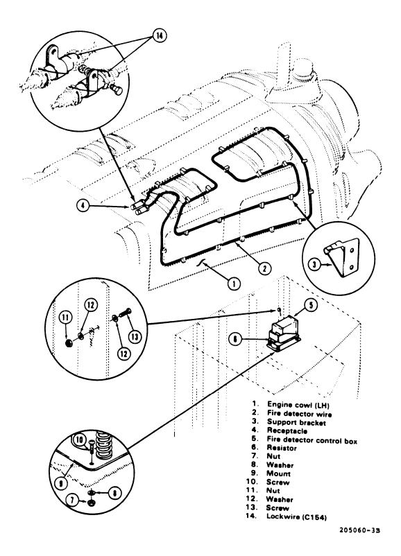
Figure 12-1. Engine Fire Detector
