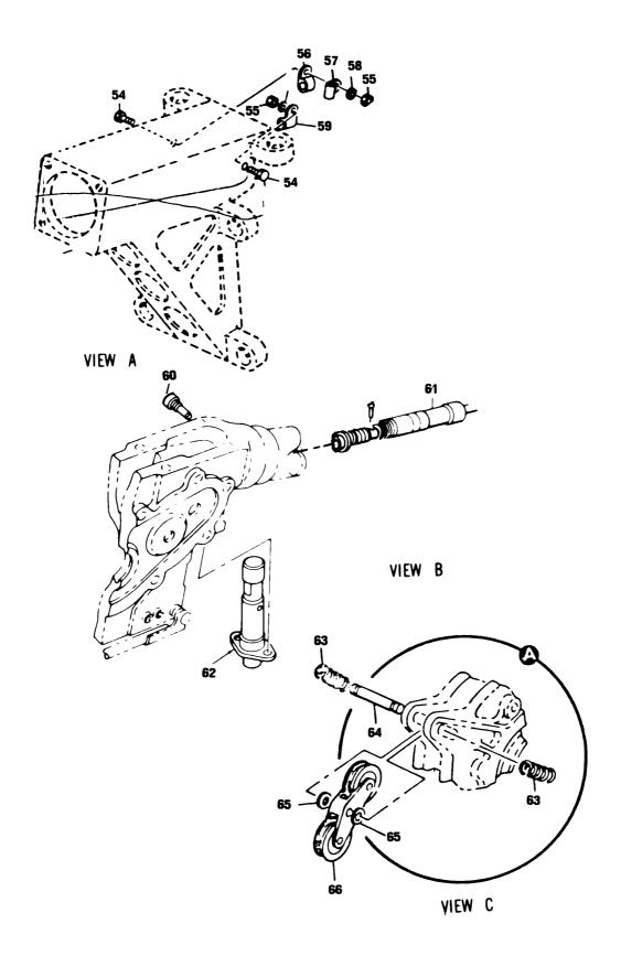
Figure 14-22. Boomhead Assembly (Sheet 2 of 4)
