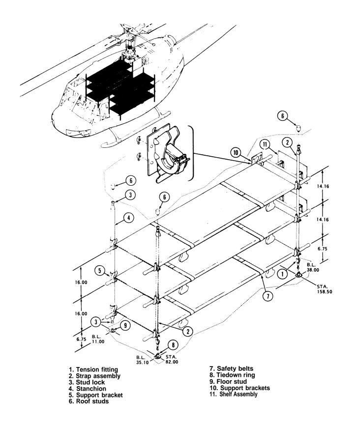
Figure 16-3. Litter Rack Installation (6 Litters)
