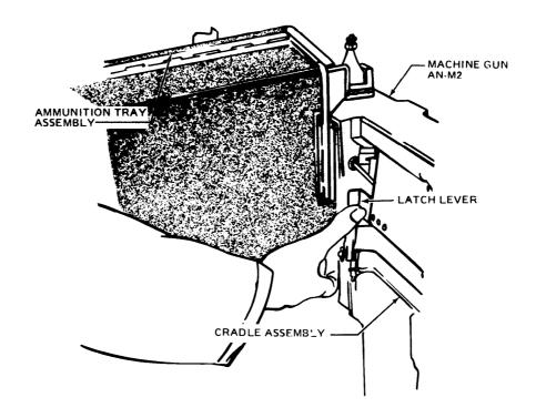
Figure 16-24. Installation/Removal of Ammunition Tray Assembly
