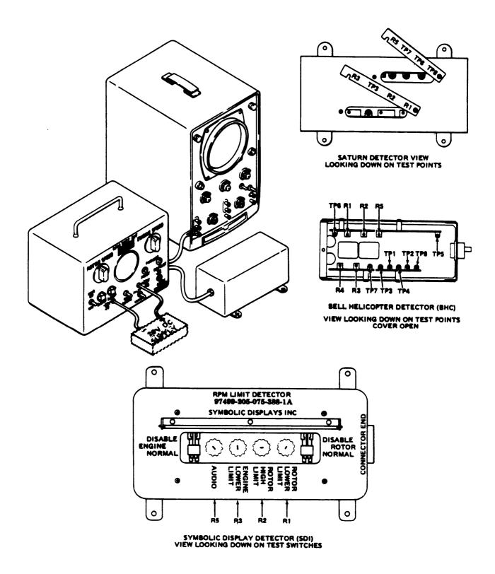
Figure 9-10. Bench Test Set Up for BHC Model, Saturn Model, and SDI Model Rpm Limit Warning. Detector
