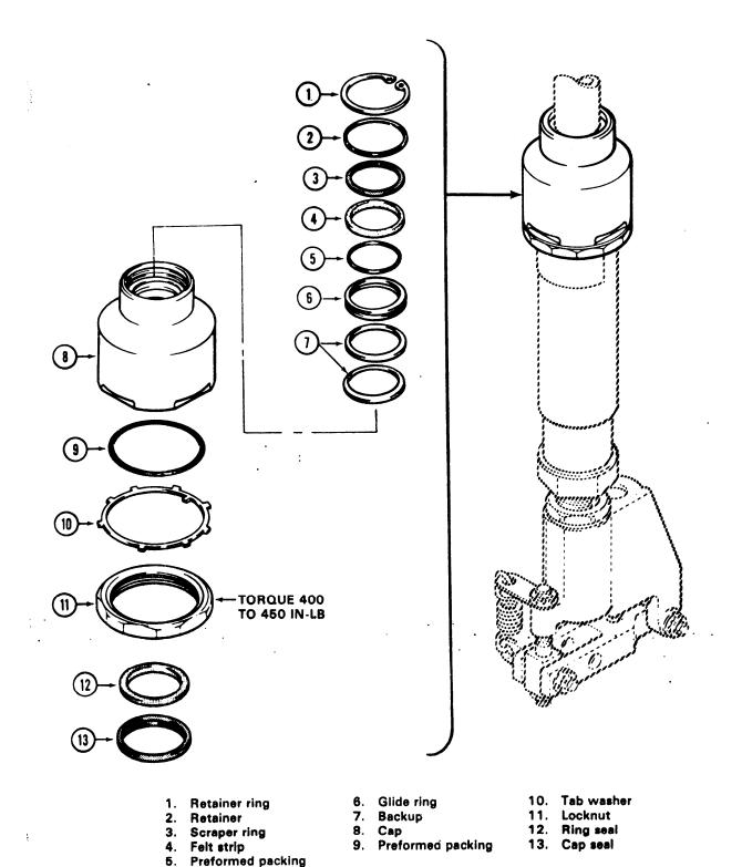
Figure 7-15. Hydraulic Cylinder Assembly P/N 100585-1 - Disassembly and Assembly
