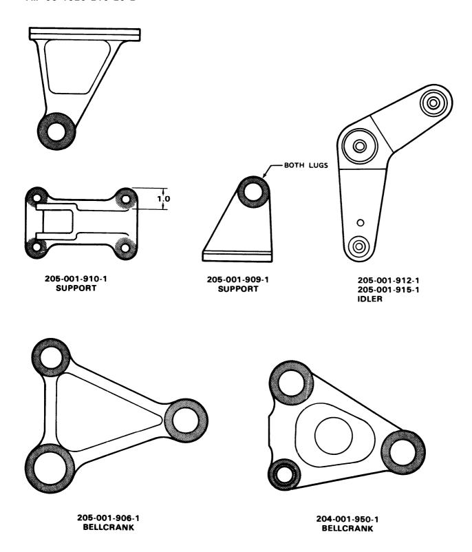
Figure 11-43. Wear and Damage Limits (Bellcranks, Levers, and Supports) — Elevator Control System (Sheet 2 of 3)
