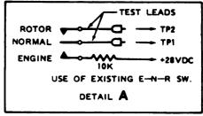
Figure 9-9. Cables for Alignment of Rpm Limit Warning Detector
