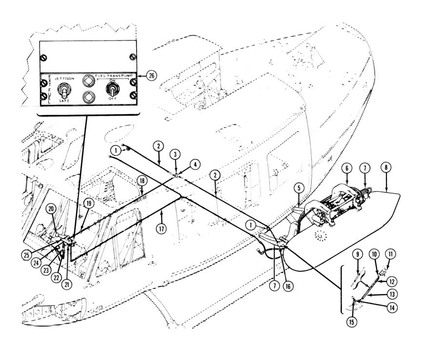
Figure 16-2. Manual Release Mechanism (Sheet 1 of 2)
