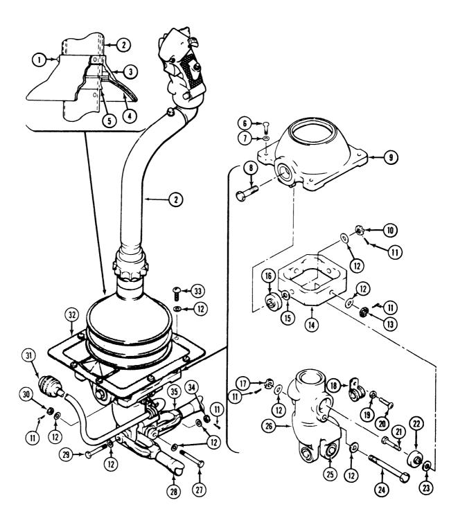
Figure 11-13. Cyclic Control Stick Assembly (Sheet 1 of 2)
