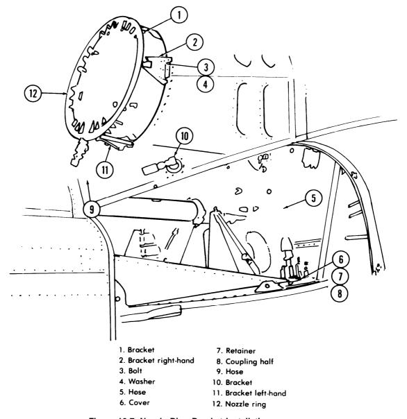
Figure 16-7. Nozzle Ring Bracket Installation
