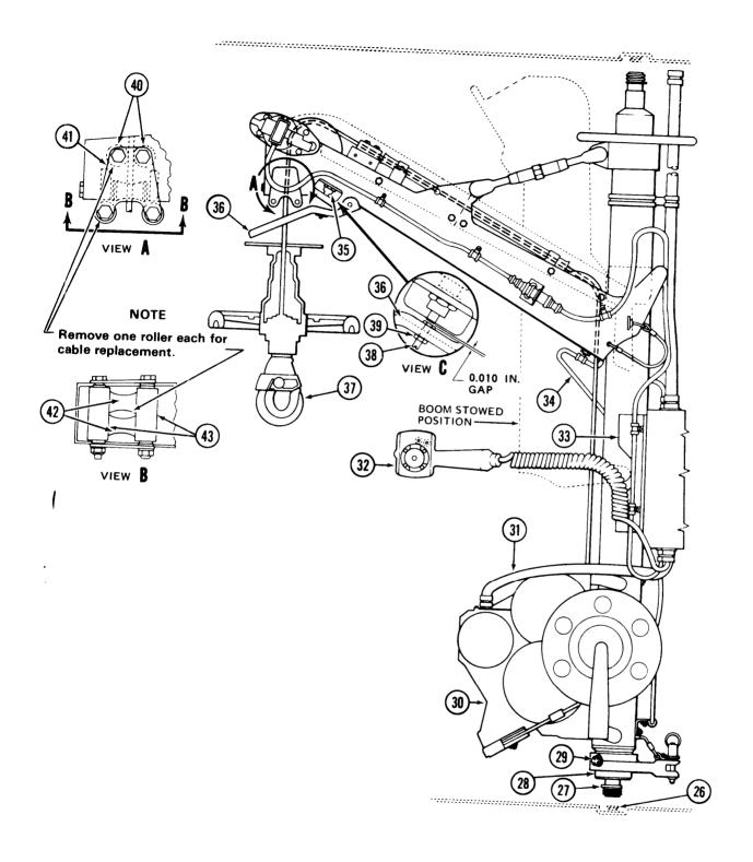
Figure 14-1. Rescue Hoist (Sheet 2 of 3)
