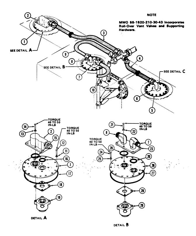
Figure 10-2. Rollover Protection Vent Valves — Aft Fuel Cells (Sheet 1 of 2)
