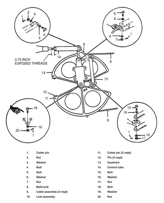
Figure 11-30. Quadrant Assembly — Tail Rotor Controls — Removal and Installation (Sheet 1 of 2).
