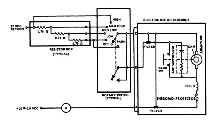
Figure 12-6. Electric Motor Assembly - Schematic Diagram
