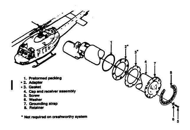
Figure 10-11. Closed Circuit Refueling Receiver.
