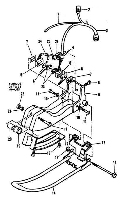
Figure 14-24. Cable Roller, Guide, and Up-Limit Switches
