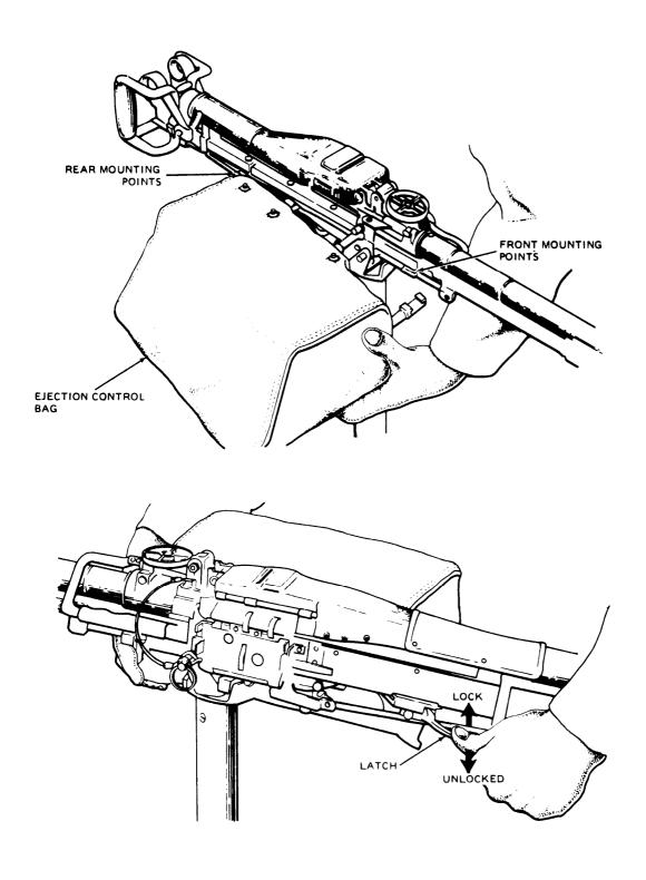
Figure 16-17. Ejection Bag Removal and Installation
