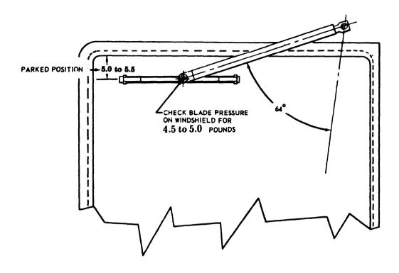
Figure 12-8. Testing Windshield Wiper
