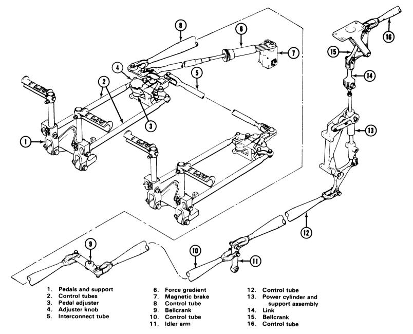
Figure 11-24. Tail Rotor Control System (Sheet 1 of 2)
