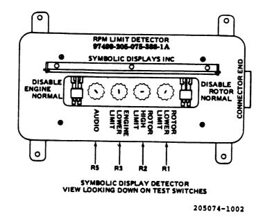
Figure 9-8. SDI Model Rpm Limit Warning Detector
