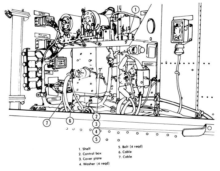
Figure 16-6. Control Box Installation
