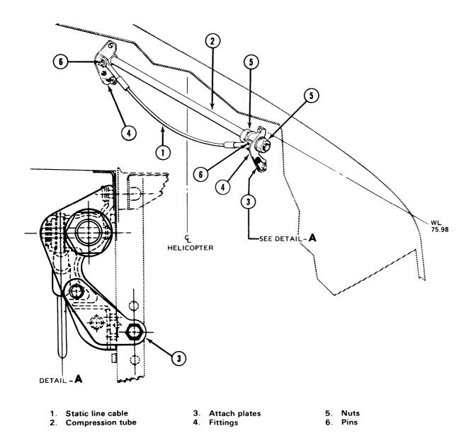
Figure 16-39. Paratroop Static Line Cable
