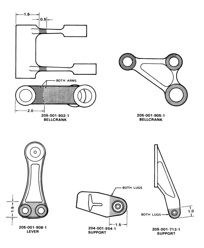
Figure 11-43. Wear and Damage Limits (Bellcranks, Levers, and Supports) — Elevator Control System (Sheet 1 of 3)
