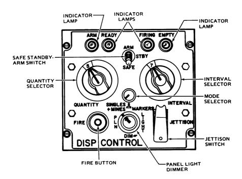
Figure 16-29. Mine Dispenser Control Panel
