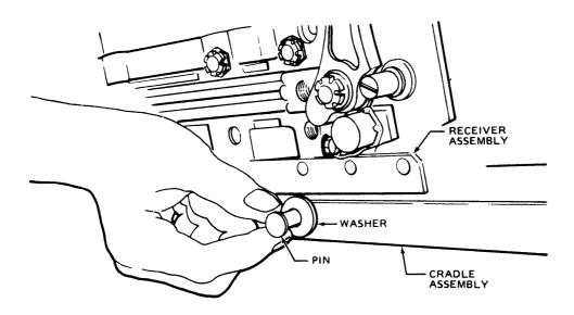
Figure 16-26. Installation/Removal of Caliber .50 Machine Gun XM213
