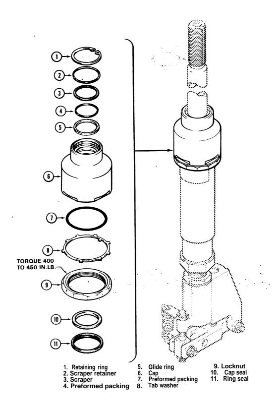
Figure 7-16. Hydraulic Cylinder Assembly P/N 100585-7 — Disassembly and Assembly
