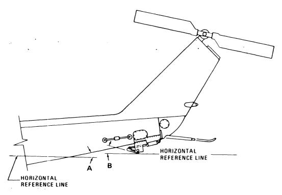
Figure 9-17. Extend Limit Switch Alignment
