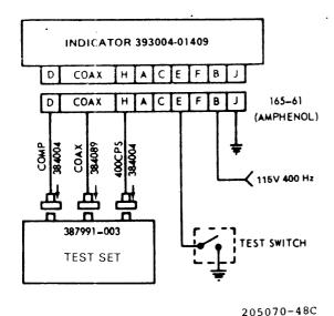
Figure 8-6. Indicator Bench Test Circuit (Crashworthy)
