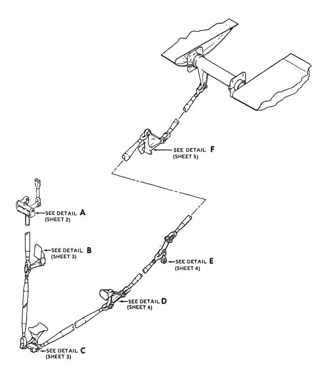
Figure 11-41. Elevator Controls System (Bellcranks, Levers, Supports, and Control Tubes) — Removal and Installation (Sheet 1 of 5)
