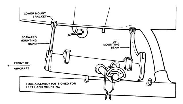
FORWARD AND AFT MOUNTING BEAMS - LOWER MOUNT BRACKETS
