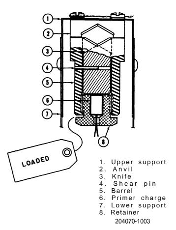
Figure 14-9. Guillotine Assembly and Support
