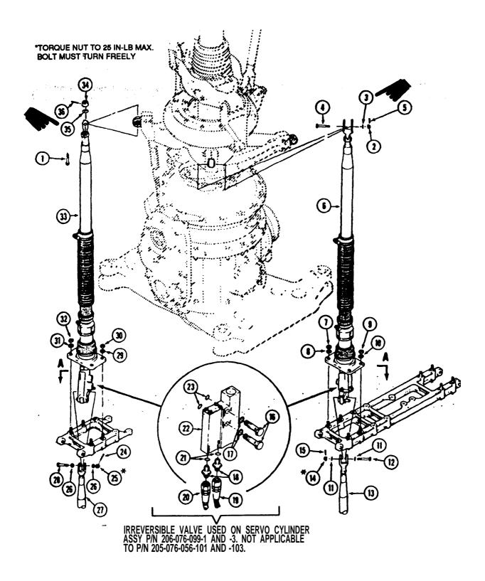
Figure 7-11. Hydraulic Cylinder Assemblies Fore and Aft and Lateral Cyclic Controls-Removal and Installation (Sheet 1 of 4)
