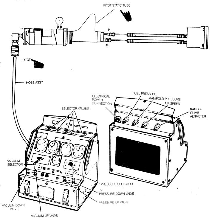
Figure 8-1.1. Connection for Pitot Leak Check (Typical)
