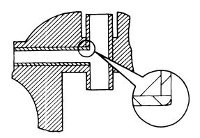
Figure 11-13.7 Corner Wear on Insert (PM 21265)
