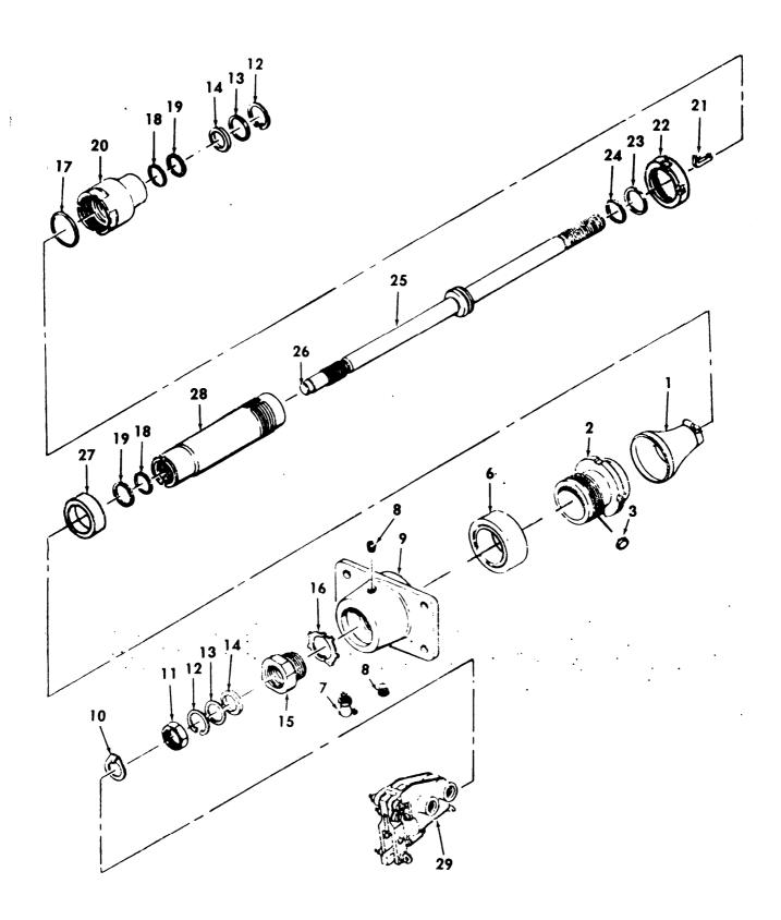
Figure 7-14.1 Hydraulic Cylinder Assembly P/N 205-076-099
