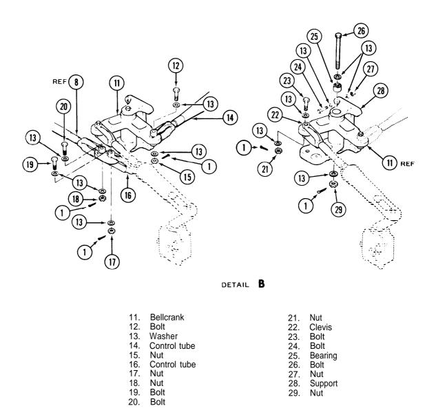
Figure 11-21. Cyclic Control System (Bellcranks, Levers, Supports, and Control Tubes) – Removal and Installation (Sheet 2 of 5)
