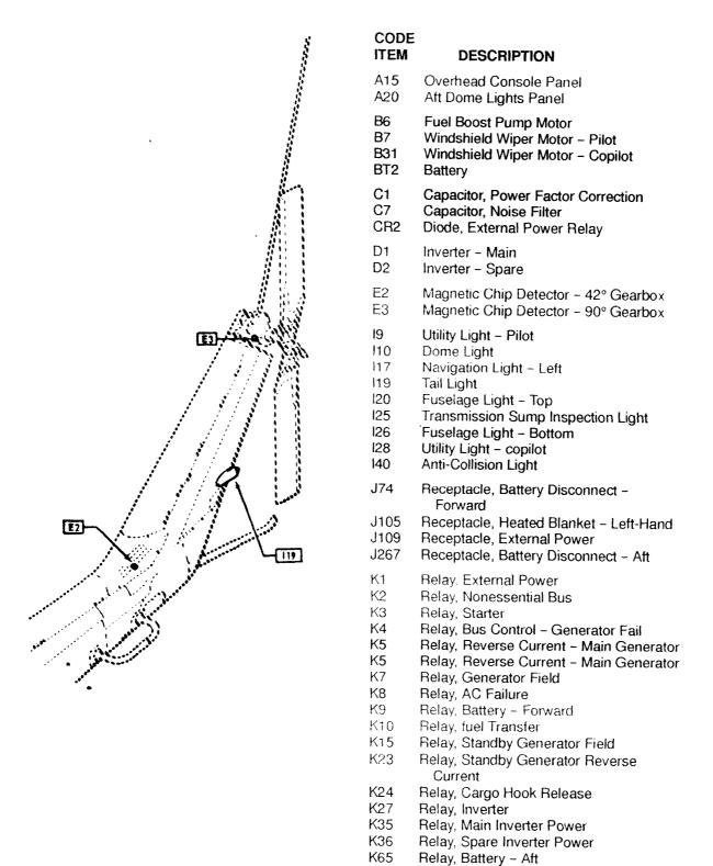
Figure 9-2. Electrical Equipment Location (Sheet 2 of 3)
