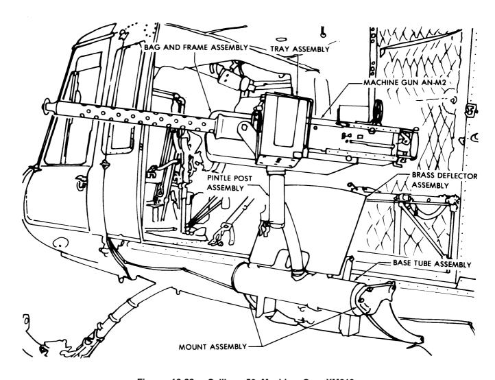
Figure 16-22. Caliber .50 Machine Gun XM213
