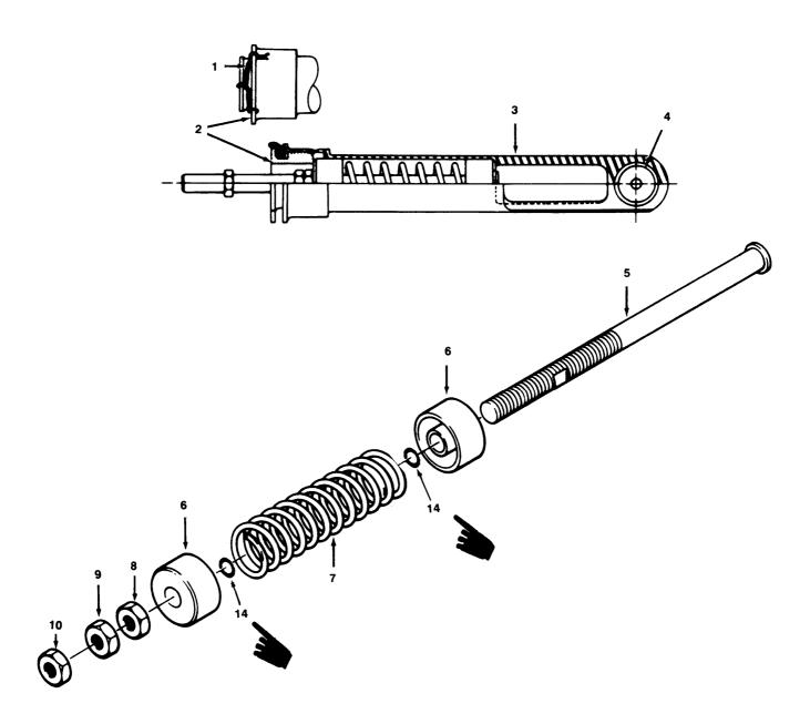
Figure 11-16. Force Gradient Assembly Adjustment (Sheet 1 of 2)
