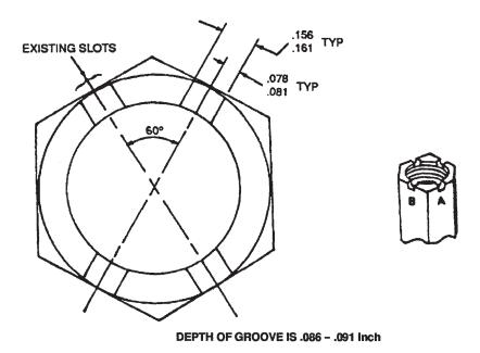
Figure 7-23.1. Additional Slots in Tube Assembly
