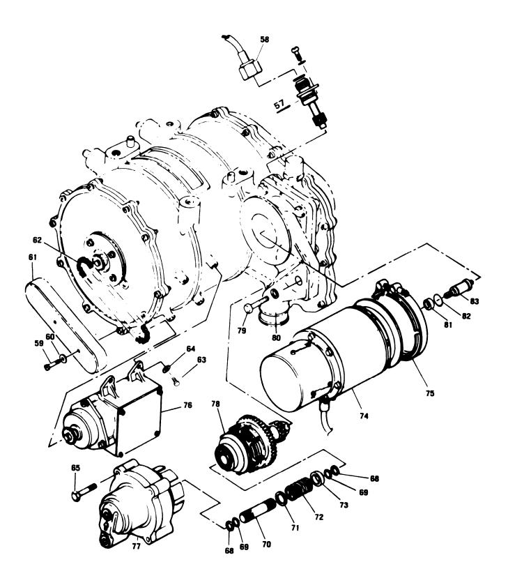
Figure 14-16 Hoist AssembLy, Parts Location (Sheet 2 of 3)
